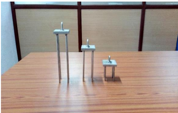
Fig .1 Model pile group of L/D ratios 10, 20 and 30
